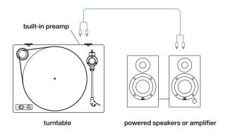
With the built-in preamp enabled, you can connect your Orbit directly to powered speakers or an amplifier using the included RCA cables.
