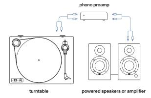
If your Orbit doesn't have a built-in preamp, you can connect it to a standalone phono preamp then connect to powered speakers or an amplifier.
